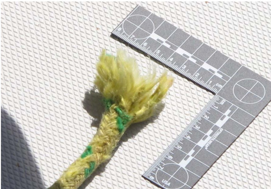
Figure 13: Picture bitter end of the parted towline.
