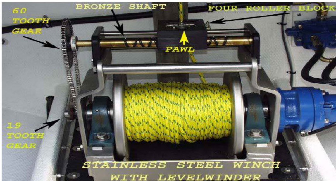
Figure 7: Picture of a winch similar to the winch onboard the M/V X-TREME.
