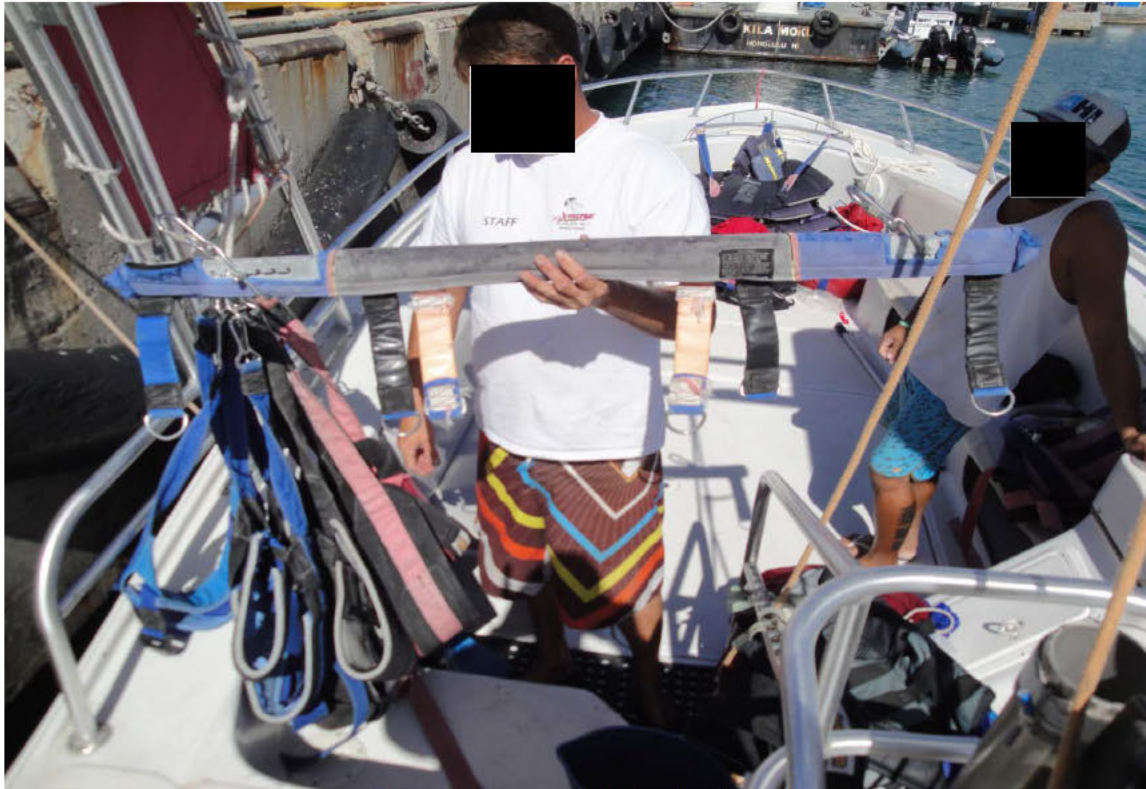
Figure 6: Picture of M/V X-TREME triple bar similar to the tandem bar that was lost.
